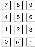
**Number Key Pad** is used to enter numeric values. The +/- key is used to enter positive or negative angles in the multi state mode.
